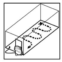
Position the Compass<sub>TM</sub> machine in the door way, lock front casters. Start at furthest point in the room and work towards the door.
